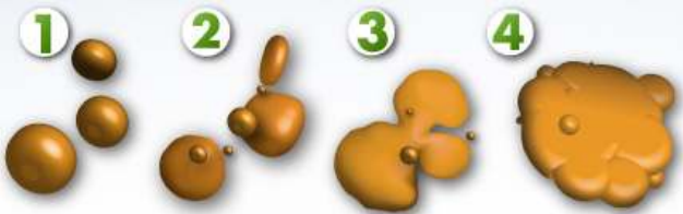
Cavitation at microscopic level
